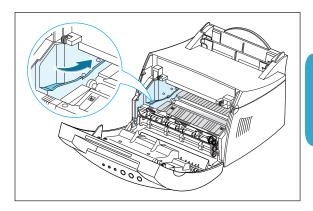
5 Grasp the handle and insert the cartridge in the printer until it snaps into place.
